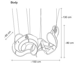
On-site adjustable overall length: 130-170 cm On-site adjustable overall height: 100-140 cm
